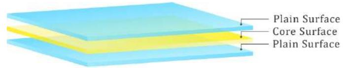
**KEY FEATURES** - SPARSHPET-LL is High Clarity, balanced shrinkage, excellent machinability film with both side plain surfaces. The film possesses good thermal, mechanical, optical and surface properties along with excellent transparency and Dimensional stability.
